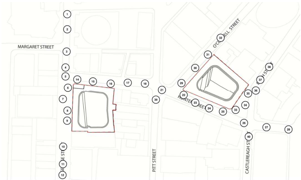
Figure 2-8 Irwin probe assessment locations for the base case (layout was provided by FJMT) which shows the layout of the two developments and the surrounding environment
